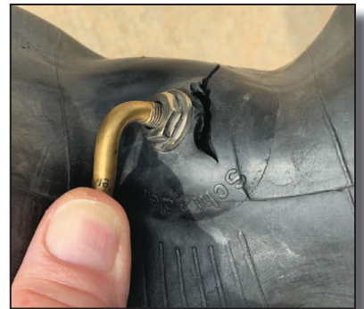
Under inflated aircraft tire upon landing resulted in tube failure at the valve stem base.
